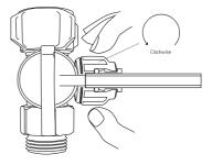
4. Once the tube is secured in position, turn the quick connect nut clockwise to secure.
