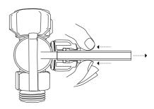
6. Push the collet against the quick connect nut and slide tube out of fitting.
