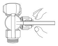
3. The fitting grips before it seals. Ensure the tube is pushed all the way into the tube stop.
