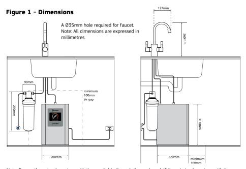
Note: Ensure there is adequate ventilation available through the cupboard. If there is inadequate ventilation, and the cupboard temperature rises to above 40°C, the system may become damaged and malfunction which will void the product warranty. To ensure there is sufficient cross-flow ventilation suitable holes or vents will need to be cut into the cupboard and door.
