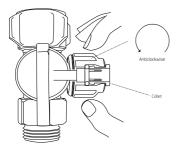
Turn the guick connect nut on the SmartTee™ anticlockwise to release the collet.
