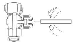
2. Cut the tube square and push into into the tube stop (inside the collet). For metal tube; remove burrs and chamfer tube end to prevent O-ring seal being damaged.
