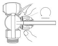
5. Turn the quick connect nut on the SmartTee™ anticlockwise to release the collet.
